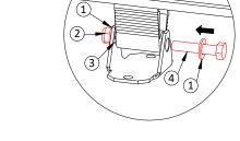
Slide the M6 Screw with install the spring Washer and fix it with a stop Nut.
