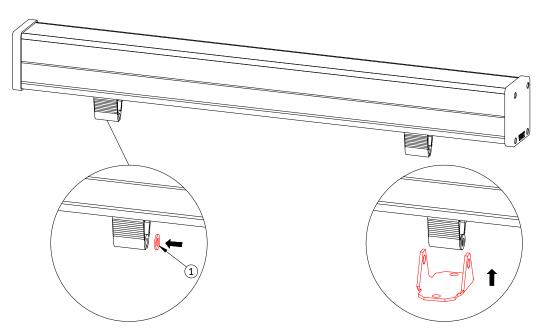
Add the polycarbonate washer provided with the fixture.
